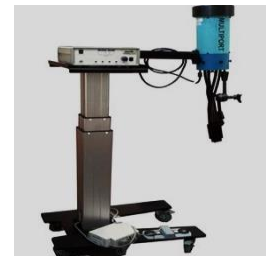
SPF Testing 601 V2.5 Multiport UV Solar Simulator
